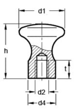
$\begin{array}{ll} d1 &= 25 \\ d2 &= M6 \\ d4 &= 14 \\ h &= 29 \\ t \ min = 9 \end{array}$
